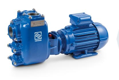
**Product Data** Suction port Threaded - 2" ISO 228 (BSP) Delivery port Threaded - 2" ISO 228 (BSP) Qmax 48 m<sup>3</sup>/h - 800 l/min (211 USgpm) Hmax 30 m (98 ft) Solids handling 25 mm (1") Motor power 4 kW - 5.5 HP Motor type **IEC** standard Winding for inverters **Cast iron frame** Motor brand WEG W22 Premium Weight 76 kg (167 lb)
